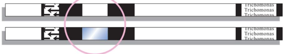
If no red Control Line appears or background color makes reading the red Control Line impossible, the result is invalid. If this occurs, repeat the test on a new Test Stick or contact Sekisui Diagnostics Technical Assistance.
