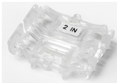
Figure 11: IN and hybridization clamps
