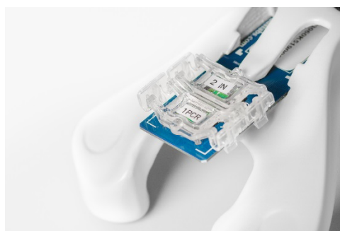
Figure 7: Sealed Chip ready for RT-PCR
