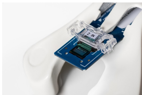
Figure 13: “2 IN” clamp attached to Chip
