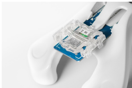
Figure 14: Sealed Chip ready for the hybridization
