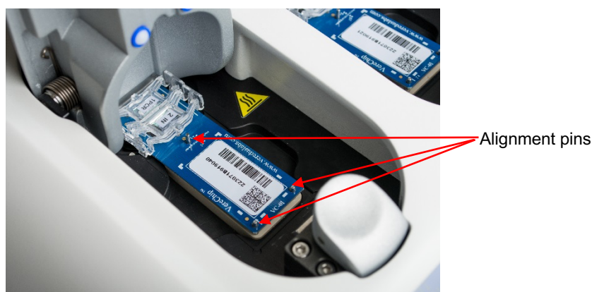
Figure 8: Chip inserted into the TCM
