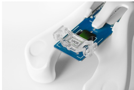
Figure 6: “1PCR” clamp attached to Chip
