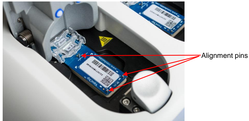
Figure 8: Chip inserted into the TCM
