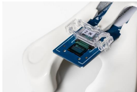
Figure 13: “ 2 IN ” clamp attached to Chip
