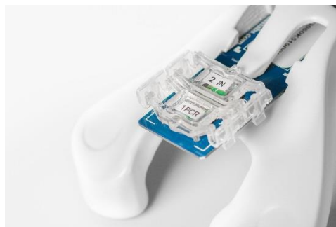
Figure 7: Sealed Chip ready for RT-PCR
