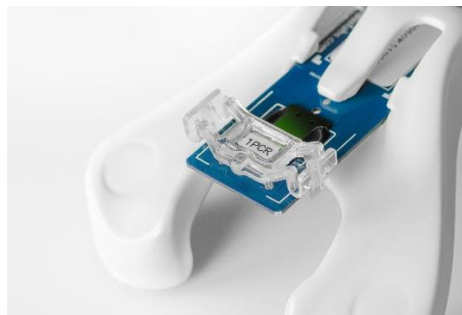
Figure 6: “1PCR” clamp attached to Chip
