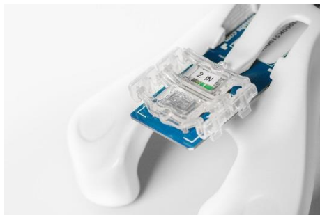
Figure 14: Sealed Chip ready for the hybridization
