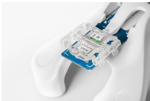
Figure 7: Sealed Chip ready for RT-PCR
