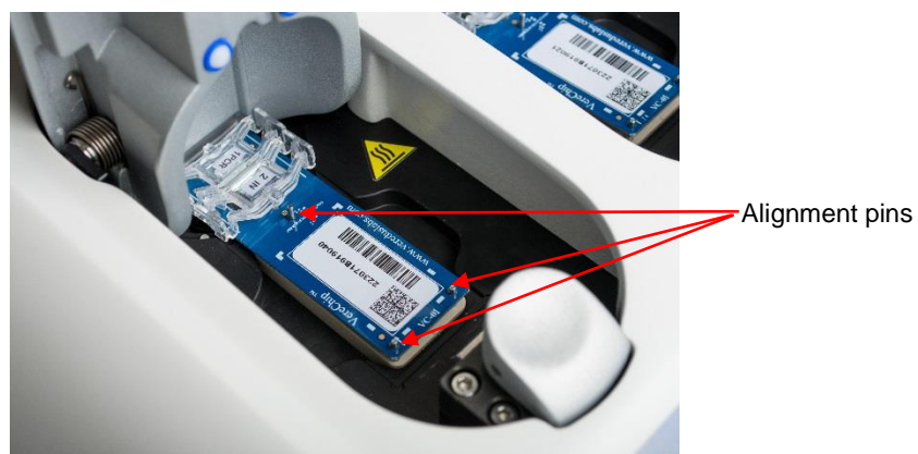
Figure 8: Chip inserted into the TCM
