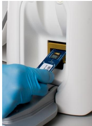
Figure 19: Chip inserted into OR
